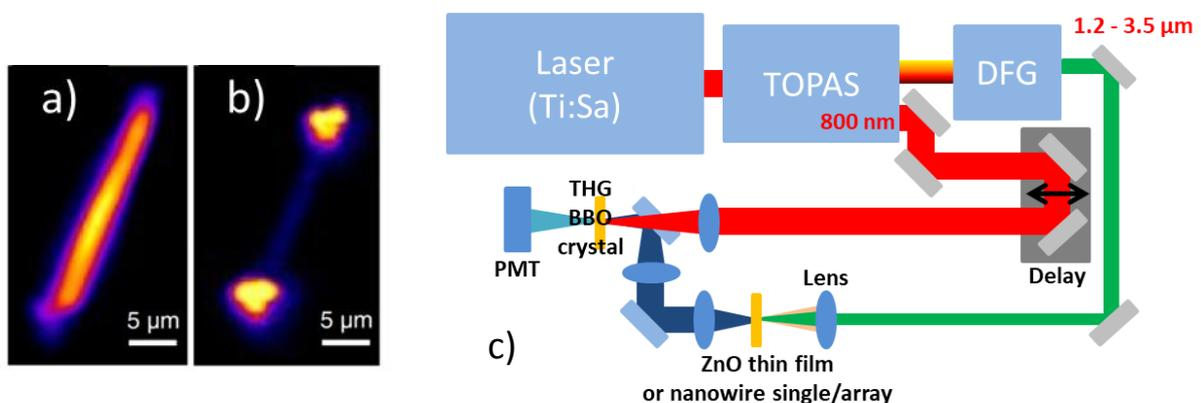
Emission profile of laser pumped nanowire a) below and b) above the lasing threshold. c) Up-conversion setup, to measure the temporal dynamic of the nanowire emission.
