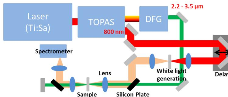
Experimental setup: The optical pump and white light probe beam are in a collinear geometry. The recombination of the two beams is realized with a silicon plate, showing high reflectivity in the visible and high transmission for the mid-IR pump pulses.
